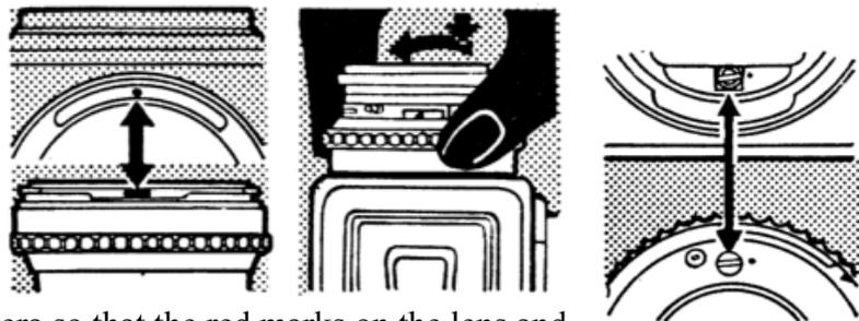
To fit the lens, mount on the camera so that the red marks on the lens and body are in line (left), then turn the lens clockwise (centre). The tensioning shafts on both the camera and the lens must have their groove lined up with the red dot before a lens can be fitted (right). This is automatically the case if the camera is always tensioned before a lens is removed or fitted.
