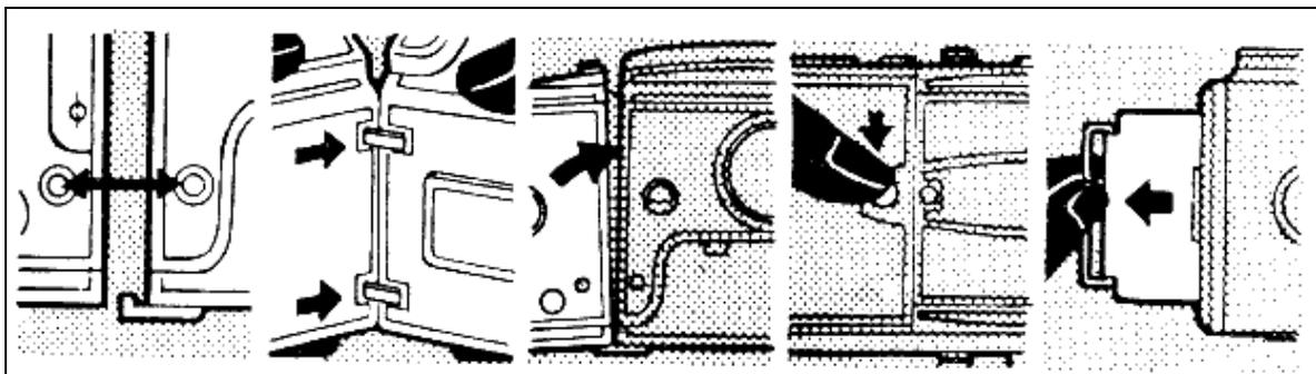
Fitting the magazine. Check that the signal on the camera and magazine correspond (left), then hook the bottom of the magazine to the camera body (centre left), push the magazine against the camera back (centre), and secure the catch (centre right). Then pull out the slide (right); the camera is now ready to shoot.
