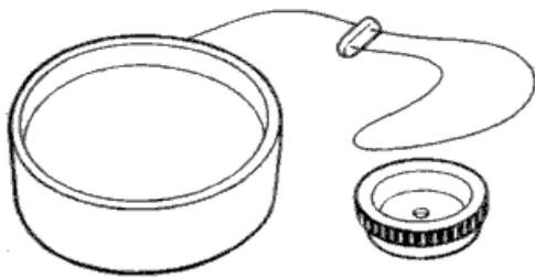
The linear mirror unit is used in photocopying when extremely accurate parallel alignment between the plane and subject is essential. It is accurate to within two minutes of arc.
