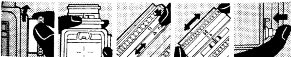
Shooting with the 500C. From left to right: Wind the film transport; view and focus the image on the screen; set the exposure value; select a suitable aperture-speed combination; press the release to expose.
