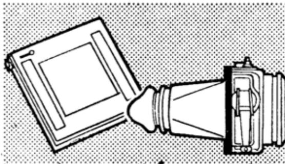
The sports viewfinder (left) fits into the shoe in the side of the camera. This finder again can be fitted with interchangeable masks for lenses of different focal length. A special version indicates the field of view for the Sonnar 150 and 250 lenses used with Hasselblads 500C/500EL and magazines A12, 12, 24 or 70.
