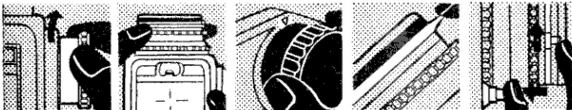
Shooting with the F models. From left to right: Wind the film and tension the shutter; view the subject on the screen and focus the lens; set the shutter speed; preselect the lens aperture; close down the lens to the preselected value and press the release.
