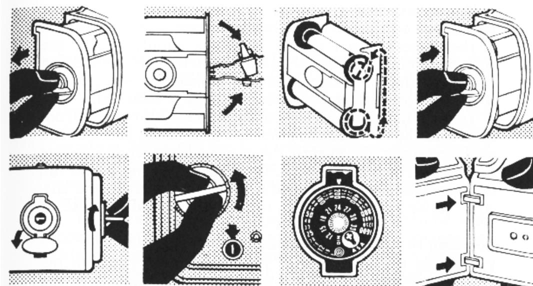
Top row: Unlock the spool holder key (left) and pull out the spool holder. Open the spool holder arms (centre left), insert the full film spool and thread the backing paper around to the empty take-up spool (centre right). Insert the loaded spool holder into the magazine and lock (right).
