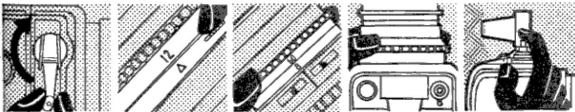
Shooting with the Super Wide C. From left to right: Wind the film transport; set the exposure value; select an appropriate aperture-speed combination focus the lens (by estimating the distances); view the subject through the wide-angle finder and press the release.
