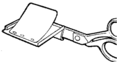
The film cutter cuts down  $2\frac{1}{2} \times 3\frac{1}{2}$  in. sheet films to  $2\frac{1}{2} \times 2\frac{1}{2}$  in. To trim the film, push it under the cover guard so it touches the stop pins. Then trim the film with the built-in scissor blades. This also must be done in total darkness.
