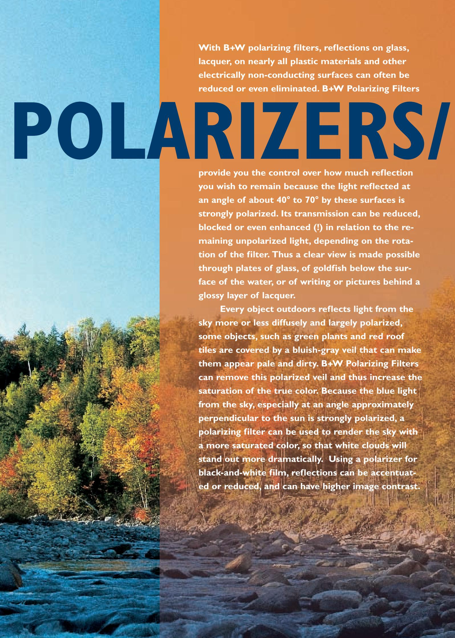
With B+W polarizing filters, reflections on glass, lacquer, on nearly all plastic materials and other electrically non-conducting surfaces can often be reduced or even eliminated. B+W Polarizing Filters
